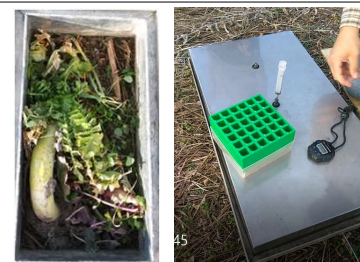
Figure 2: Example gas chamber. Field treatments were laid out at random, but gas chambers were targeted for areas that appeared representative of the treatment and included at least 1 large radish when possible (left). Sampling procedure with syringe in sampling port (right).
