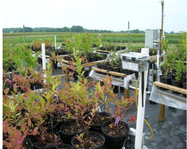
Figure 50. The AgroEcology, Inc. funded research project with wireless sensor network nodes and probes in place. Note the wireless node in the foreground.
