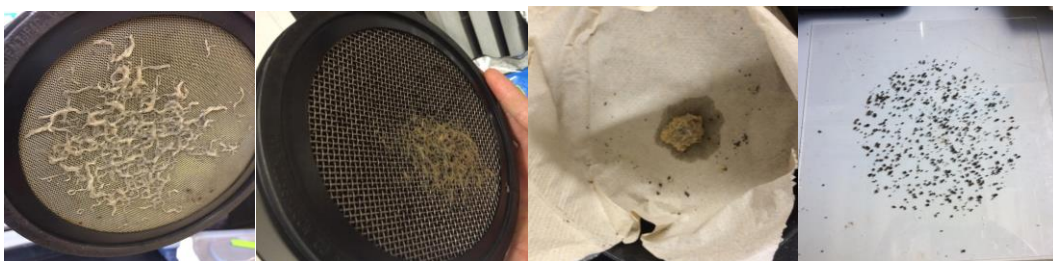
Figure 5.4. From left to right: 0.5 mm screen with high worm entanglement after 3 hrs harvesting; 2.5 mm screen with less entanglement than the 0.5 mm screen; 2.5 mm screen allowed trace amounts of soil to pass through; the amount of soil that fell through the 3.2 mm screen just after loading the sieve with soil.
